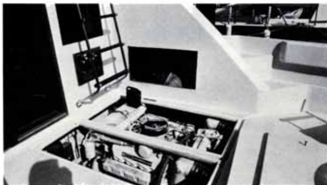
Three hatches provide engine access. Removable side panels allow man to enter and work—in this case on junction box
