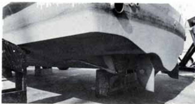
The 31' hull has broad, flat chine surfaces aft and pockets that allow for recessed stern gear and lower shaft angles
