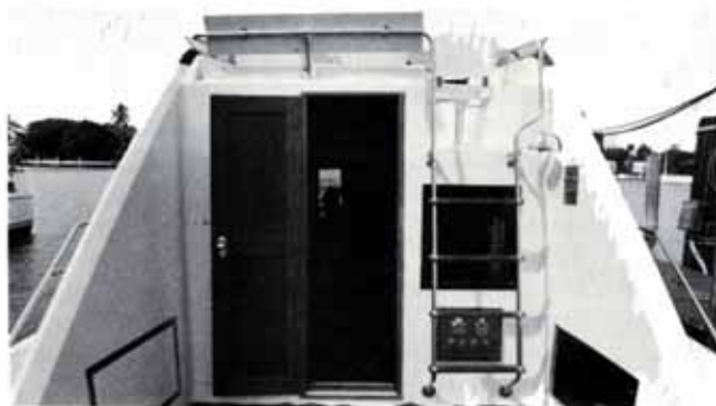
Stainless steel shore connector panel is below tinted window in cabin bulkhead. Ladder rails continue around bridge
