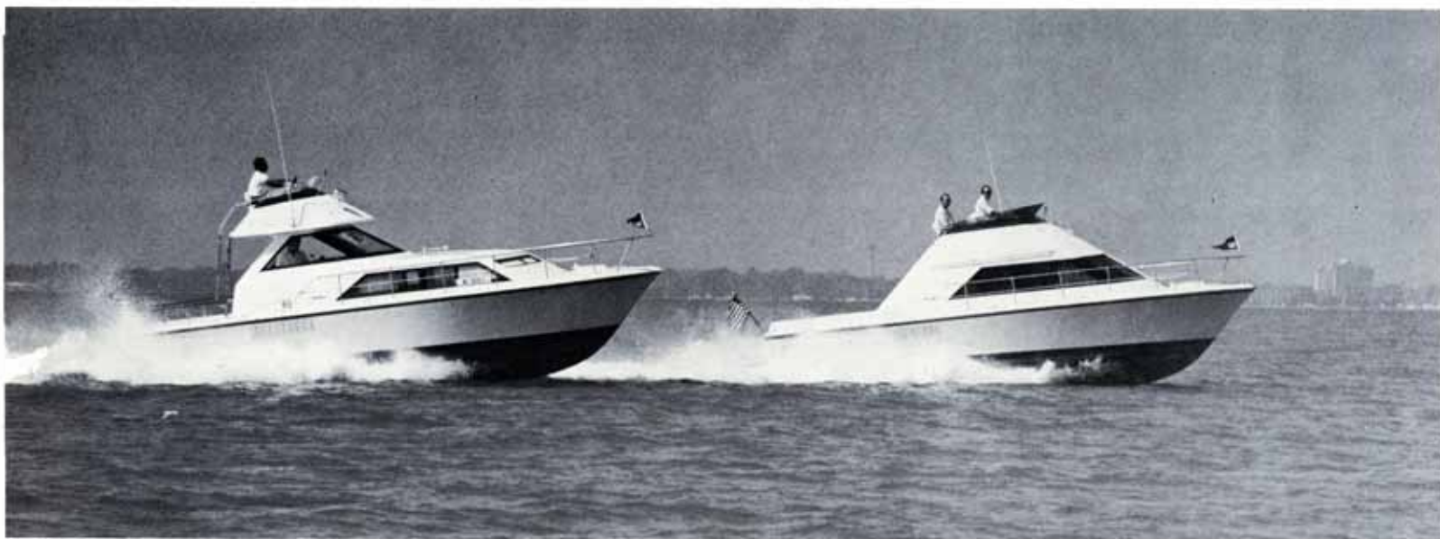
Above: Express Cruiser follows Sport Cruiser during run on Biscayne Bay. Sport Cruiser option is a second set of controls in place of convertible lounge below. Note flat running attitude
