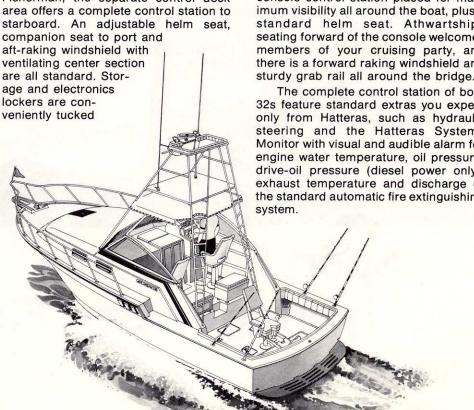
inside the wings alongside the helm and companion seats, while an optional tackle box and cooler/dunnage box can be installed aft of the seats, secure and convenient without getting in the way.
