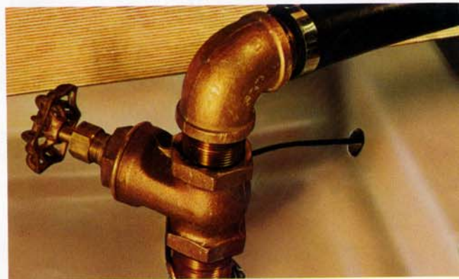
A standard on all Hatteras boats—sea valves are installed on all through-hull underwater fittings. All underwater fittings are mechanically bonded to a common ground to help prevent electrolytic erosion of metals.
