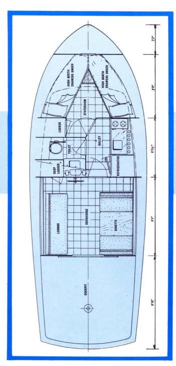
Sleeps 6 • LOA 34 ft. 2 in. • Beam 12 ft. 6 in. • Draft 36 in. • Weight 11 000 lbs. • Speeds to 40 MPH with twin 280 HP engines • 6 ft. 2 in. headroom • Dual or single controls • Fly bridge See specification sheet for options.
