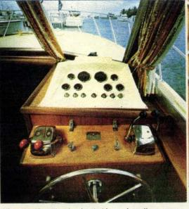
The control station in the deckhouse has all necessary instruments and switches. The full view windshield is equipped with a windshield wiper.
