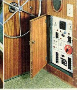
Hatteras Master Electric Panel provides central control and protection for both 12-volt and 110volt. All circuits have circuit breakers and master switches. Switches for generator and battery charger circuit. Indicator for battery condition.
