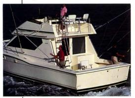
dead-rise, convex-vee Hatteras hull to a smooth lift. This hull shape is well suited to the displacement and balance characteristics of this 38' 10" machine. It tracks well into head seas, remains poised in following seas and bites into stable, maneuverable turns.
