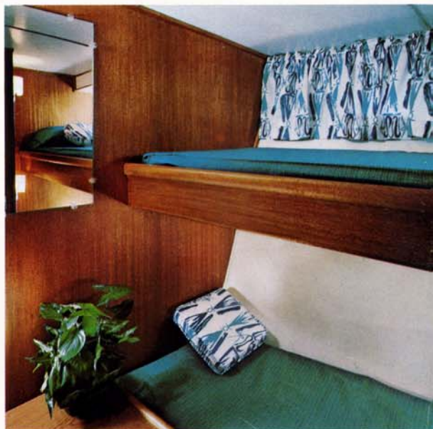
Guest stateroom has upper and lower 6 ft. 3 in. bunks with foam mattresses. 12-volt lights over each bunk. Built-in chest, hanging locker and drawer beneath lower bunk provide 17 cu. ft. storage. Mirror over chest. Floor is carpeted. Headroom is 6 ft. 3 in. Screened portlight.
