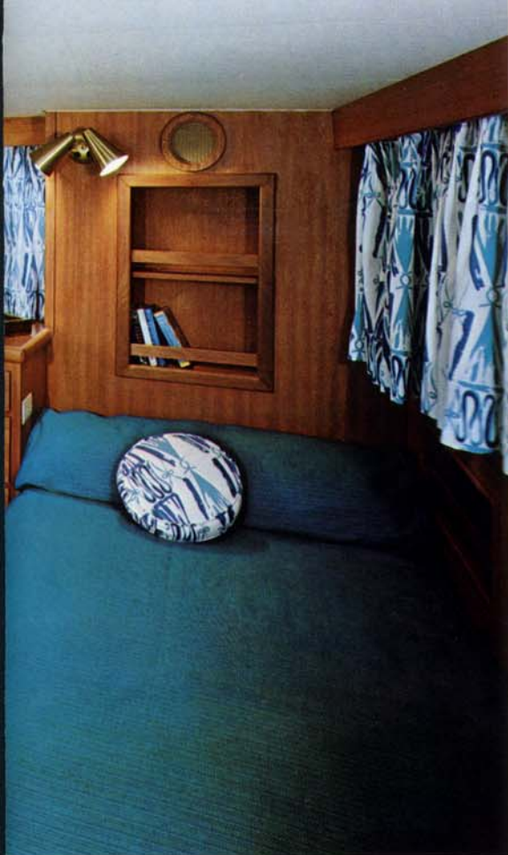
Guest stateroom has upper and lower 6 ft. 3 in. bunks with foam mattresses. 12-volt lights over each bunk. Built-in chest, hanging locker and drawer beneath lower bunk provide 17 cu. ft. storage. Mirror over chest. Floor is carpeted. Headroom is 6 ft. 3 in. Screened portlight.
