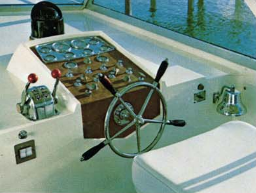
This close-up view of the control station on the bridge shows the standard equipment: Battery selector switch, single lever controls, compass. Chart deck is 6 ft. 9 in. x 8 ft. 4 in. with hatch to deckhouse companionway. There is a ventilating windshield; a hardtop with a dome light. Height on aft deck to hardtop is 6 ft. 5 in.
