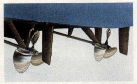
V-struts and intermediate struts keep Hatteras propeller shafts securely in alignment for maximum performance at high speeds and even in heavy seas. Underwater fittings are heavy-duty manganese bronze.
