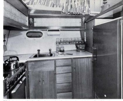
Efficient, roomy galley has three-burner electric stove and oven, ten cu. ft. refrigerator with freezer; ample dish lockers, glass rack. Plenty of storage space and drawers; stainless steel sink, exhaust blower over stove; 110 volt outlets for appliances.
