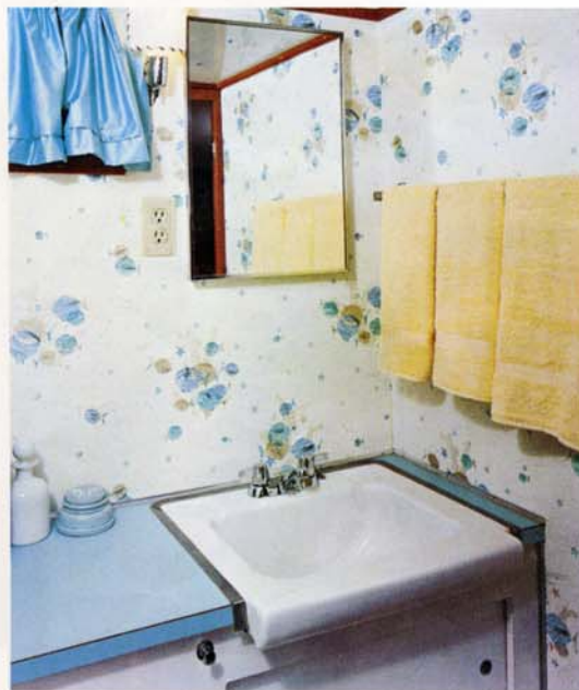
The aft stateroom head is equipped with a vitreous china lavatory and hot and cold pressure water; a 6-in.-size stall shower with curtain; large linen locker; medicine chest with mirror; storage space in vanity (has micarta top); bulkhead light and 110-volt outlets; screened portlight; towel bar and paper holder; decorator wall covering.
