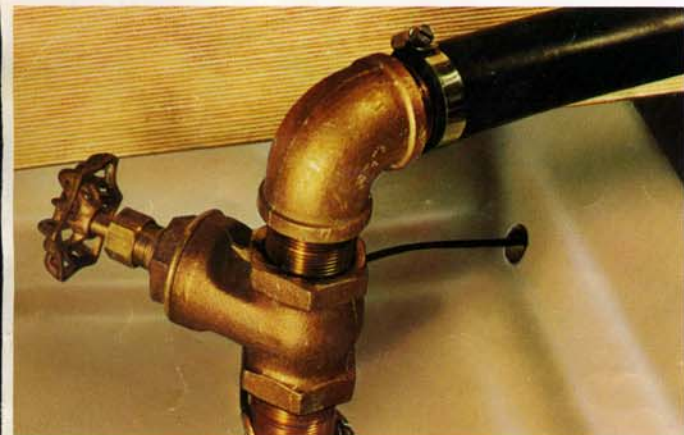
A standard on all Hatteras boats—sea valves are installed on all through-hull underwater fittings. All underwater fittings are mechanically bonded to a common ground to help prevent electrolytic erosion of metals.
