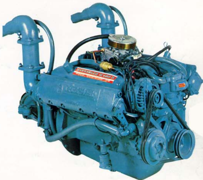
The gasoline engine option is twin 290 H.P. engines. Because of the Hatteras fiberglass construction and lack of frames, there is extra space around the engines to make them easily accessible.
