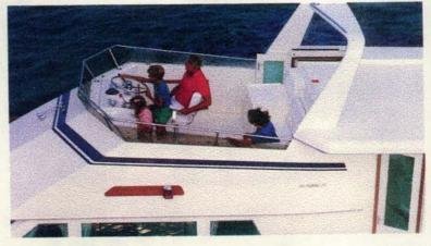
FLYING BRIDGE is constructed of molded fiberglass and includes ample storage under the control console, L-shaped lounge with storage, stainless steel rails and stanchions, and a control station with all the necessary switches and dimmable lighted instruments for operating efficiency and simplicity.
