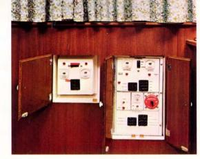
Hatteras Master Electric Panel, the last word in yacht safety and electronics. Central control and protection for both 12-volt system and 110-volt A. C. Voltage input from shore line or from generator can be read at a glance—also current being used. Battery condition is indicated. All circuits are protected by circuit breakers and master switches.
