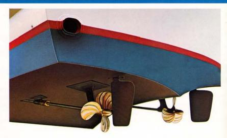
Sturdy struts and intermediate struts keep Hatteras propeller shafts securely in alignment for maximum performance at high speeds and even in heavy seas. Underwater fittings are heavy-duty manganese bronze.
