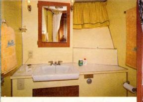
▲ The bow head has an electric toilet; a vitreous china lavatory; a medicine cabinet with mirror; shower and sump pump. There is ample storage space. Vinyl tile floor covering. Curtains on the screened port light; an exhaust blower; 110-volt outlets.
