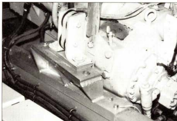
Welded aluminum engine mounts straddle glass stringers.
