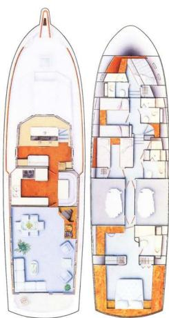
The standard layout of the Hatteras 65 Motor Yacht, shown at left, illustrates the large dressing area with vanity that is included with the master stateroom.
