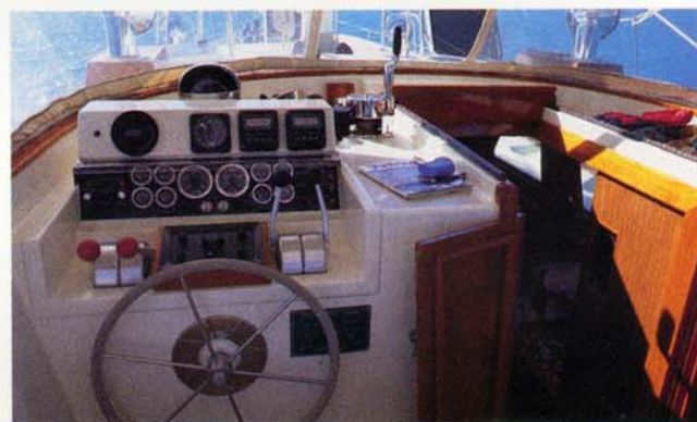
Main helmsman's station is at forward end of 65's center cockpit, protected by dodger when needed, and features full range of instruments, electronics from autopilot to radar.
