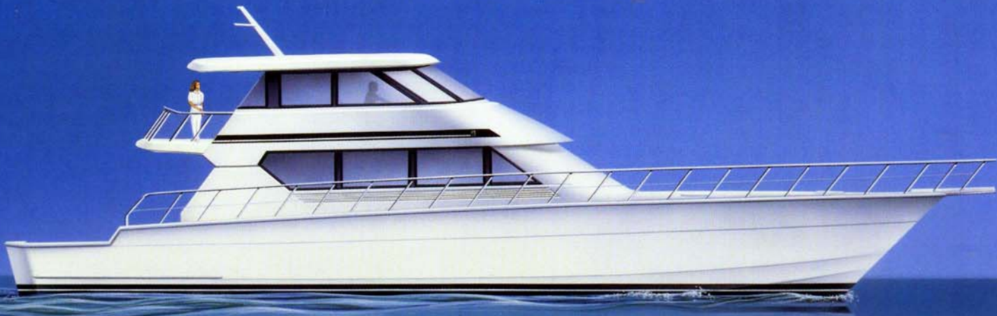
Alternate Extended Bridge Deck
